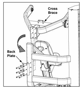
2. Secure the ARM BRACKET CROSS BRACE to the FRONT TUBING with four (M8, 20MM, Button Head Screw) and four (M8, Washers). Tighten with a 4MM hex key.
